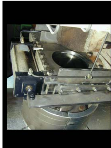
DN400 PN40 Stargate-O-Port-Valve® on wood pellet reactor capping application
