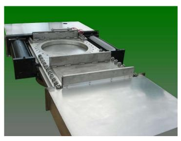
For full automation of reactor fill operations, capping valves are used instead of manually installed blanks.
