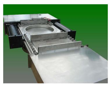
For full automation of batch digester fill operations, capping valves are used instead of manually installed blanks.
