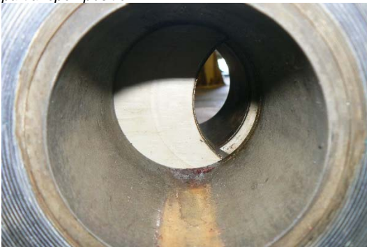
Scale removed without damage to sealing surface
