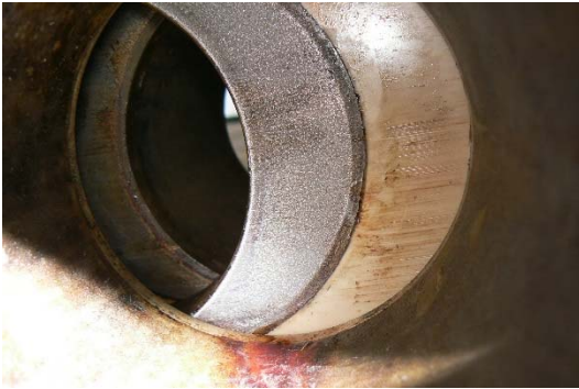
Example of metallic scale formation. Valve in service in partial open position
